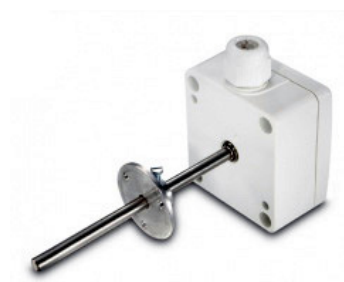
260 0636 PT100 Air-duct sensor, 1/3 DIN, 4-wire
